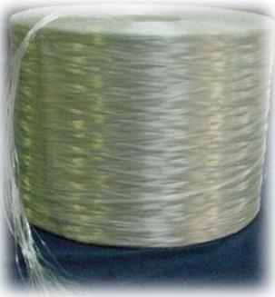
**EICOSPRAY - 687**, Spray-up Roving is produced with **E-CR** glass filament strands, gathered together into a single bundle and wound on a cylindrical package without twist and with even tension. The Glass filaments are coated with a proprietary silane sizing system and have fast resin impregnation with good air release properties.
